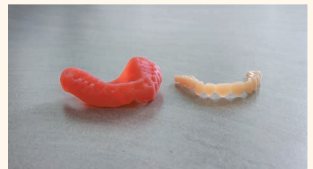
Fig. 9: 3D-printed base and milled teeth without supports.
