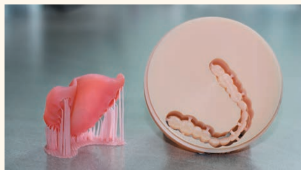
Fig. 8: 3D-printed base and milled teeth with supports.
