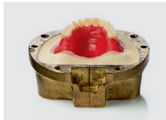
2. Filling the flask with the wax-up
