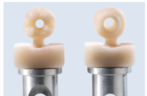
Fabrication of one-piece/multi-piece abutments from hard block materials
