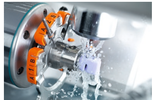
Grinding in the carving mode reduces processing times by up to 60%
