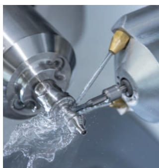
Wet machining of a titanium abutment blank using the "rotary milling" technique
